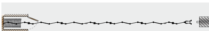
Impacco singolo a scomparsa Stacking to one side with stack in custom build box
